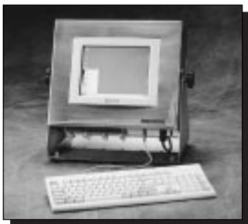
A standard PS/2 style keyboard can be quickly attached via an external keyboard port.
